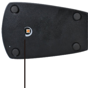
Adjustment of the microphone Gain
