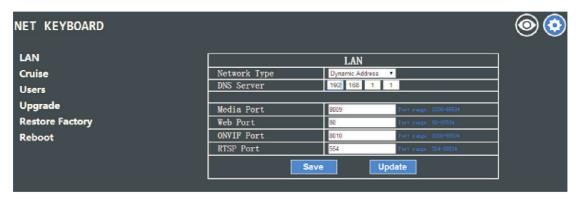
Dynamic addresses (the default): The keyboard will automatically request an IP address from the router and it can be displayed on the keyboard after the request is successful, the format is "Local IP: 192.168.x.xxx".
